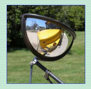
See children in blind spots Shows area to the front or side of the bus hidden from direct view Use the grid! Adjusted for each driver □ Ask mechanic for help □ It's the law! Check crossovers last at every stop "Rock 'n Roll" to see in the mirrors
